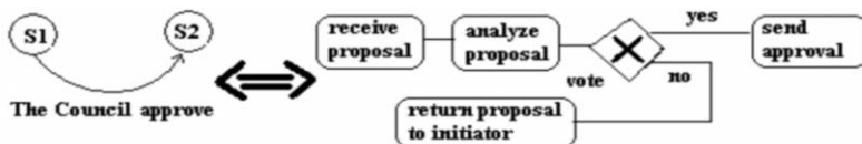
Figure 3. Two equivalent models (at left, a social network and at right, a BPMN diagram, for the administrative process “Approval by the Council”)
